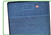
Battery is charging
